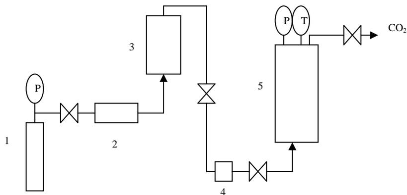
**Figure 1** - Supercritical CO<sub>2</sub> treatment system. 1, CO<sub>2</sub> cylinder; 2, filter; 3, Cooling bath; 4, high-pressure plunger-pump; 5, reactor (thermostat of the pressure vessel). The labels T and P refer to the temperature probe and the pressure gauge, respectively.
