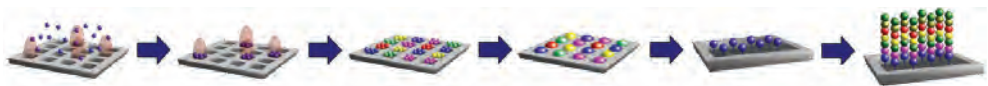
Fig. 1. Left to right: Solid phase peptide synthesis on CMOS chips: Negatively charged micro particles containing amino acids are guided to their synthesis sites by the selectively programmable electric fields of the CMOS chip, particles containing one specific sort of amino acids are deposited, particles containing all sorts of amino acids for the first layer of the peptide array are deposited, heating initiates the coupling of the first layer of amino acids to the surface, remnants of particles and excess amino acids are discarded in chemical washing, repeating this procedure leads to a complete peptide array (From Beyer et al. (2007). Reprinted with permission from AAAS.)
