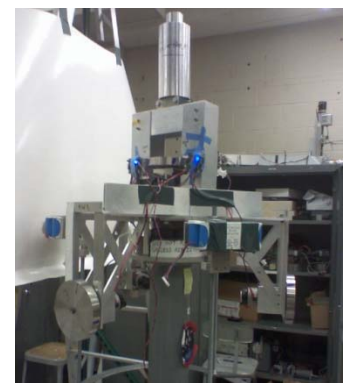
Fig. 4: ACS with installed Protection/CM Mount.
