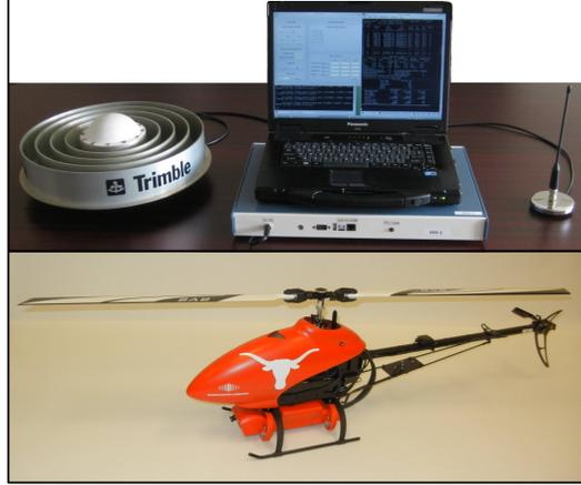
Figure 11: Spoofer hardware and target RUAV.
