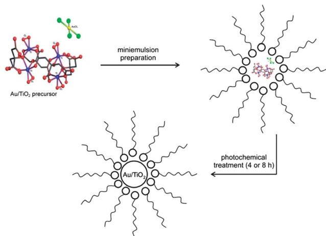
**Scheme 1** Formation of Au/TiO<sub>2</sub> nanocomposite in miniemulsion by photolysis of AuCl<sub>4</sub>(NH<sub>4</sub>)<sub>7</sub>[Ti<sub>2</sub>(O<sub>2</sub>)<sub>2</sub>(cit)(Hcit)]<sub>2</sub> · 12H<sub>2</sub>O.
