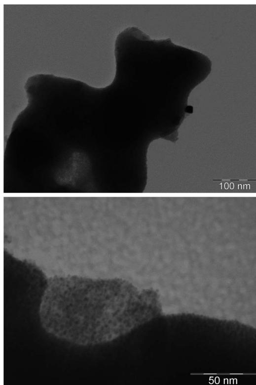
**Fig. 2** TEM micrographs of the Au/TiO<sub>2</sub> nanocomposites: (top) T100-4 and (bottom) T100-8.
