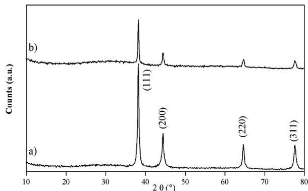
**Fig. 1** XRD patterns of Au/TiO<sub>2</sub> nanocomposites: (a) T100-4 and (b) T100-8.
