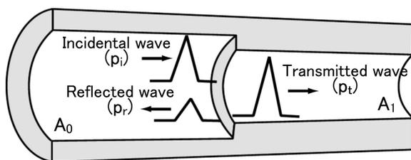
Fig. 2. Reflection and transmission of acoustic waves at a boundary where cross-sectional area discretely changes. The amount of reflection and transmission of an acoustic wave is calculated by a reflection coefficient,  $r = (A_0 - A_1)/(A_0 + A_1)$  where  $A_0$  and  $A_1$  are the cross-sectional areas leftward and rightward of the boundary.
