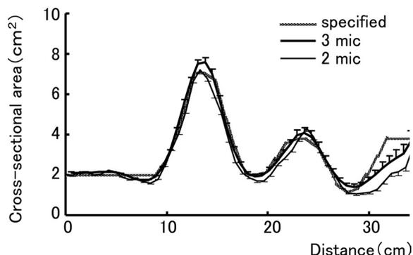
Fig. 4. Comparison of the estimated cross-sectional area between this and the conventional 2-microphone method. Data are means + SD (3-mic) and means - SD (2-mic) of 50 measurements. In this method, both reflection coefficients  $r_0$  and  $r_1$  were set as 0.00. Mean cross-sectional areas by this method coincided with those by the conventional method with slight differences in extreme values and in the further distances >20 cm. SD was not different between the 2 methods.
