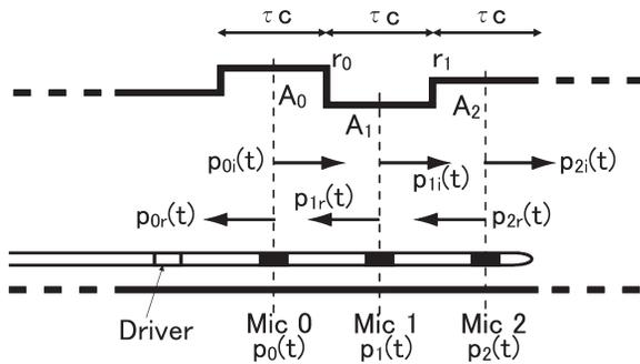
Fig. 1. Airway model to infer the reflection coefficients ( $r$ ) at microphone (Mic) positions. The cross-sectional area ( $A$ ) was assumed to be constant for an interval during a unit transmitting time ( $\tau$ ) of sound wave with a speed of  $c$ , and discretely change at its boundaries. Microphones were set in the middle of three consecutive intervals. The relationship between the observed acoustic waves with microphones and reflection coefficients  $r_0$  and  $r_1$  was formularized.
