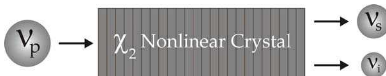
Fig. 1. The generation of long wavelength light through parametric frequency down-conversion. Here, \nu_p = \nu_s + \nu_i .
