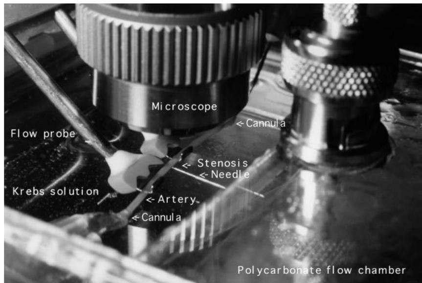
FIG. 1. Details of the polycarbonate flow chamber with the artery inside.
