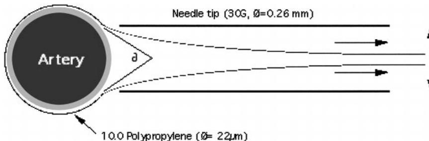
FIG. 2. Profile of the progressive arterial stenosis system used.
