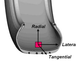
FIGURE 6. COORDINATE SYSTEM FOR THE TIRE
