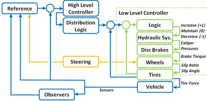
FIGURE 1. OVERALL STRUCTURE OF CONTROL SYSTEM
