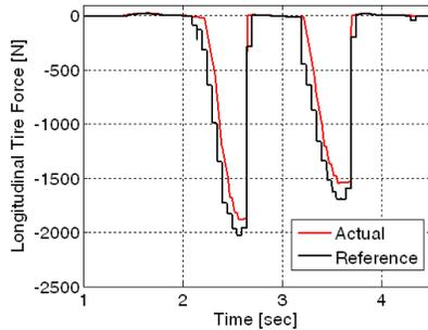
FIGURE 5. FORCE BASED FEEDBACK CONTROL
