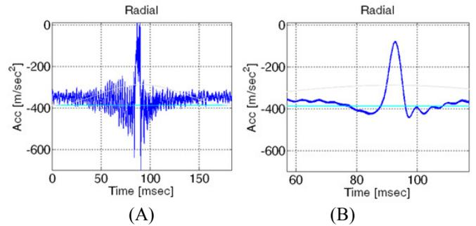
FIGURE 7. RADIAL ACCELERATION SIGNALS (A) BEFORE AND (B) AFTER LOW PASS FILTERING
