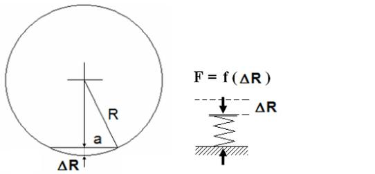
FIGURE 8. MAXIMUM RADIAL DEFLECTION AND NORMAL FORCE ESTIMATION
