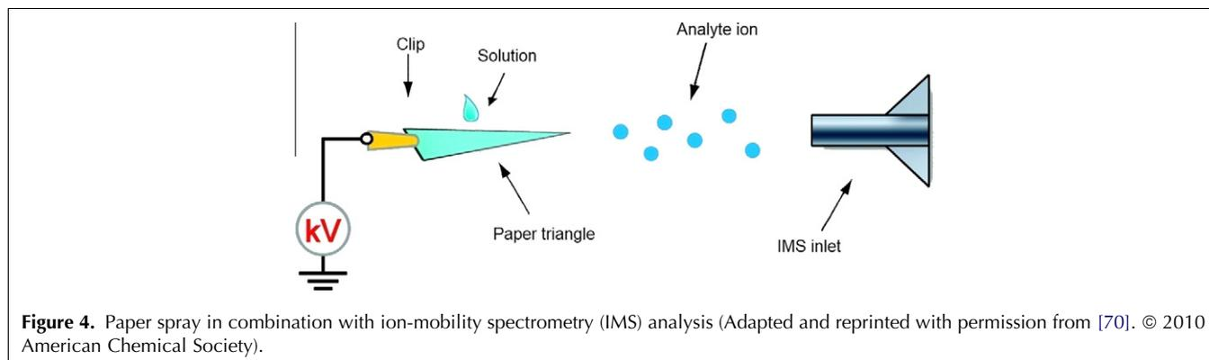
**Figure 4.** Paper spray in combination with ion-mobility spectrometry (IMS) analysis (Adapted and reprinted with permission from [70]. © 2010 American Chemical Society).
