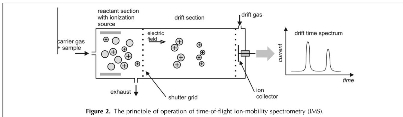
Figure 2. The principle of operation of time-of-flight ion-mobility spectrometry (IMS).
