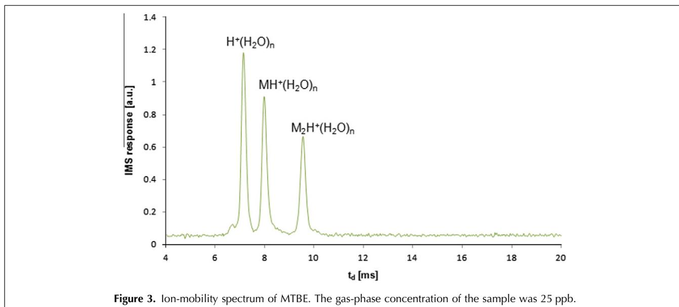
Figure 3. Ion-mobility spectrum of MTBE. The gas-phase concentration of the sample was 25 ppb.
