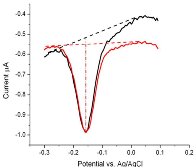
**Figure S3.** Square wave voltammetry in the presence of a non-specific antibody, measuring H<sub>2</sub>O<sub>2</sub> production for two representative cases: (black) QCM with DNP-functionalized polymer brushes and photosensitizer not exposed to antibodies (red) the functionalized QCM after exposure to the non-specific antibody. Experimental conditions were similar to those in Figures 3 and S6.
