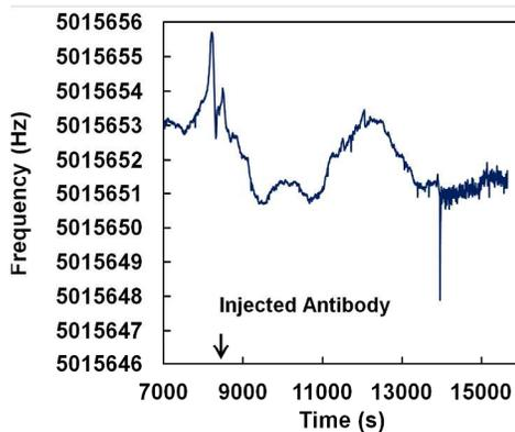
**Figure S2.** QCM frequency response to the addition of 100  $\mu\text{L}$  of 1 mg/mL non-specific sheep IgG antibody (resultant concentration, 11 nM) to a 60 mL solution of PBS, pH 7.2 containing 1 mg/mL BSA solution at 25°C. The solution was stirred throughout the measurement.
