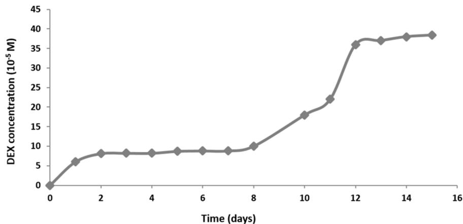
**Figure 2.** Concentration of DEX released to phosphate buffered saline (PBS) from RADA 16-I peptide hydrogel mixed with  $4 \times 10^{-3}$  M DEX in the parallel system of a perfusion bioreactor, measured each day for 15 days. Measurements were obtained by UV-Vis spectrophotometry.
