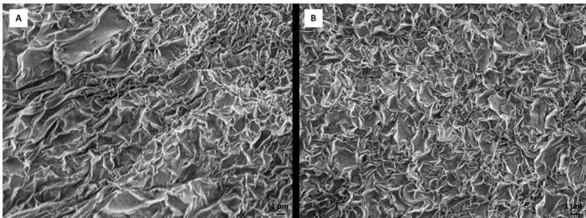
**Figure 1.** Scanning electron microscopy (SEM) images of 0.5% RADA 16-I peptide hydrogel 24 h after hydrogel polymerization, (A) without dexamethasone and (B) with dexamethasone. Scale bar represents 1  $\mu\text{m}$ .
