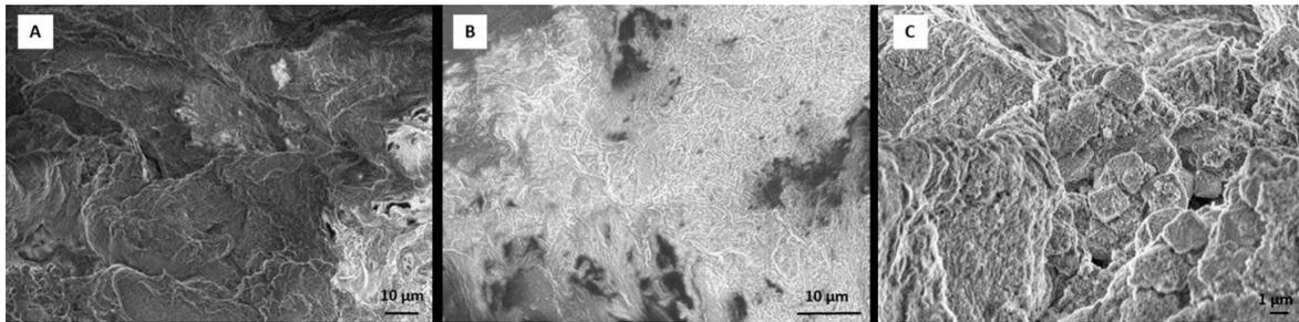
**Figure 6.** SEM images of engineered tissue on DEX-loaded RADA 16-I scaffold after 21 days of cultivation. Three morphologies that have characteristics of (A) cells; (B) extracellular matrix/connective tissue and (C) minerals can be observed. Scale bar (A,B) = 10 μm. Scale bar (C) = 1 μm.
