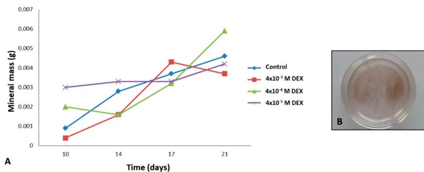
**Figure 5.** (A) Mass of deposited minerals in grams released from DEX loaded RADA 16-I scaffolds to media collected during the 21 days of culture in a perfusion bioreactor. (B) Presence of minerals in collected media confirmed with von Kossa staining.
