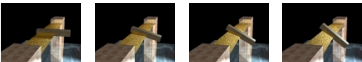
Figure 6 Sequential images showing a conceptual torsion force in a strip element.
