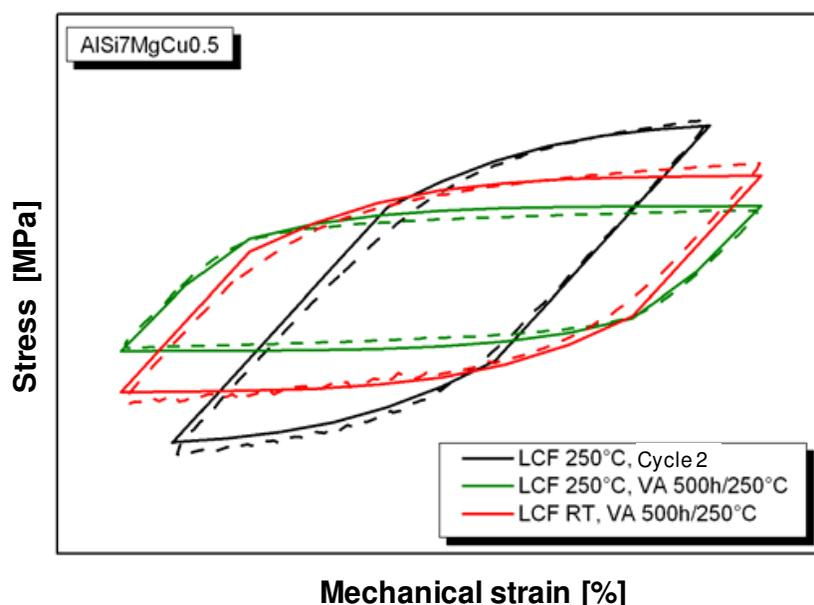
Fig. 8. Comparison of calculated and measured hystereses
