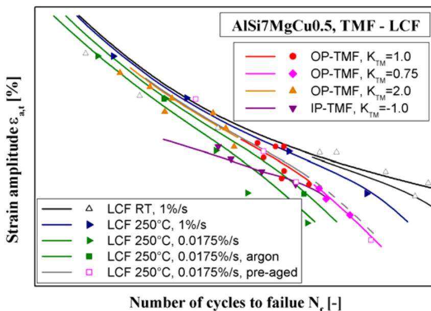
Fig. 10. Fatigue life computing under LCF, OP-TMF, and IP-TMF loading according to the Sehitoglu damage model
