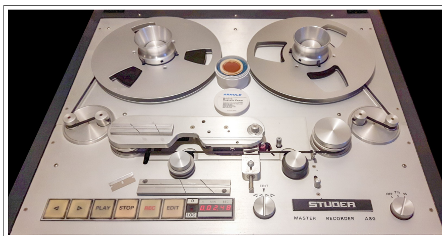
Figure 2. Studer A80-RC tape machine with an Arnold B-1022 Magnetic viewer at the ready and an EdiTail splicing block.
