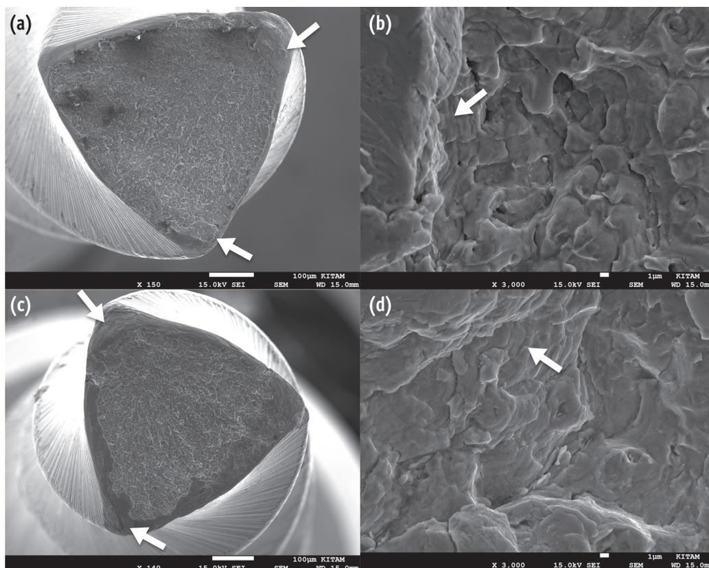
**Figure 2.** SEM appearances of the ProTaper Universal retreatment D1 files after cyclic fatigue testing. (a) and (c) General view of D1 instrument with fatigue zones, and an overload fast fracture zone (white arrows); (b) and (d) High-magnification view of D1 instrument showing fatigue striations typical of cyclic fatigue (white arrows). (a) and (b) Rotary motion group; (c) and (d) Adaptive motion group.
