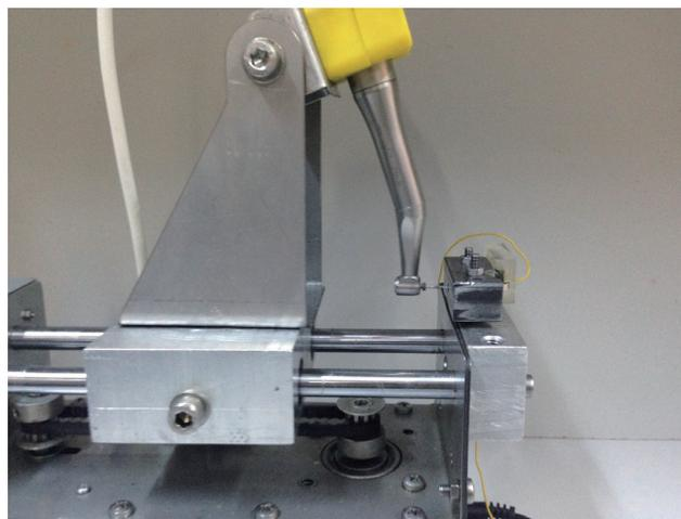
Figure 1. Dynamic cyclic fatigue testing device.
