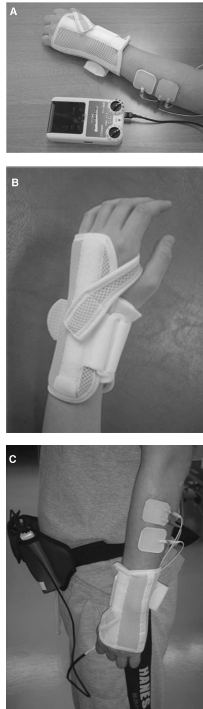
Figure 1 An Integrated Volitional Control Electrical Stimulator (IVES) Combined With a Wrist-Hand Splint
