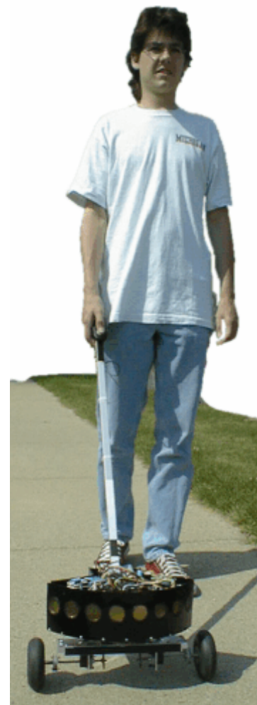
Figure 10: The actual GuideCane prototype.
