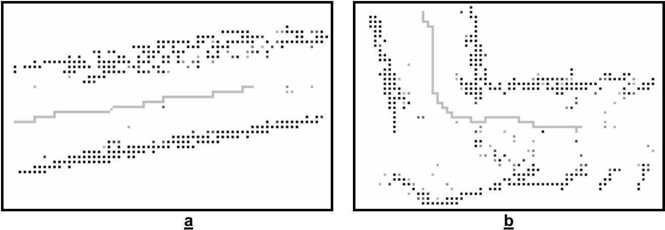
Figure 11: Two screen captures showing the path of the actual GuideCane through corridors. In both experiments the target direction is towards the right. The dots indicate filled cells in the histogram grid. Cell with a higher Certainty Value are darker. The continuous gray line indicates the GuideCane's trajectory, based on its odometry. a). The GuideCane moves along a straight corridor. b) The GuideCane makes a left turn at a T-shaped intersection
