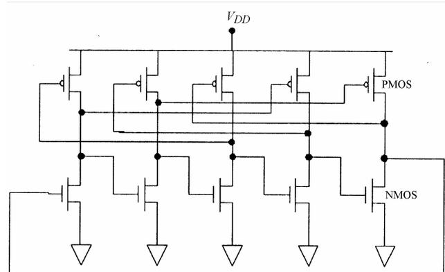
Fig. 2 — Five stages negative skewed delay ring oscillator
