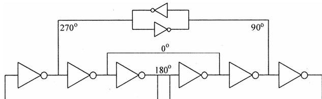
Fig. 5 — Two sets of quadrature output coupled ring oscillator based on single ended delay stages
