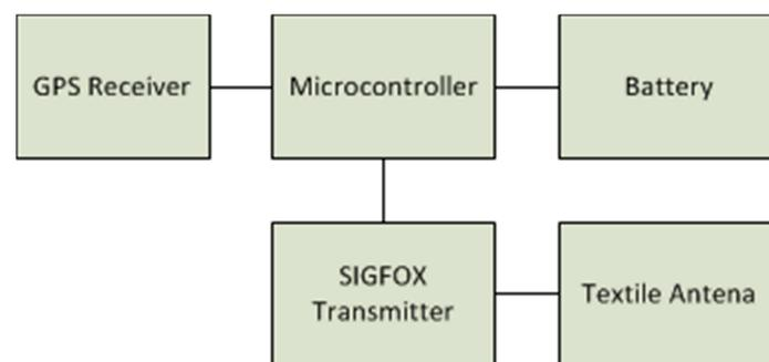
**Figure 3.** Block diagram of the proposed wireless wearable sensor node.
