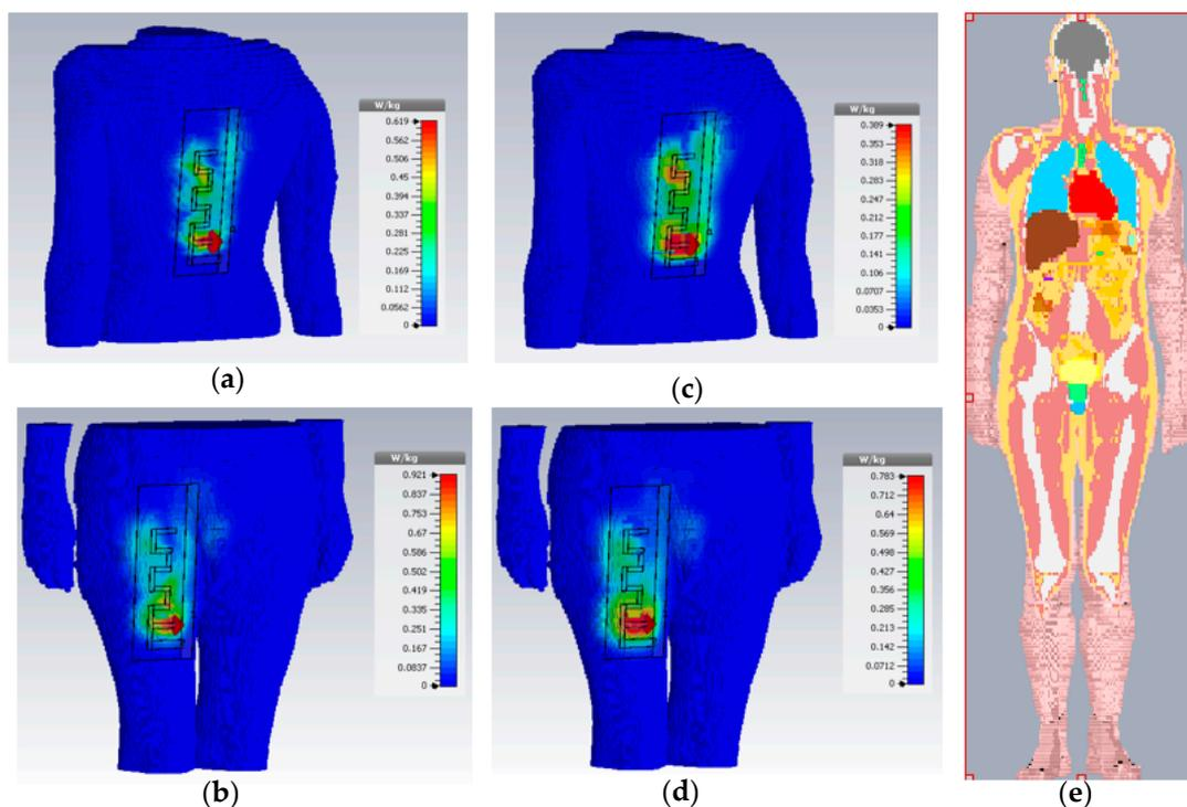
**Figure 12.** On-body jeans MIFA antenna 3D specific absorption rate (SAR) distribution at 868 MHz averaged over 1 g (a,b) and 10 g (c,d) tissue. The antenna has been located in the back and leg of a 38 year male voxel model called Gustav (e).
