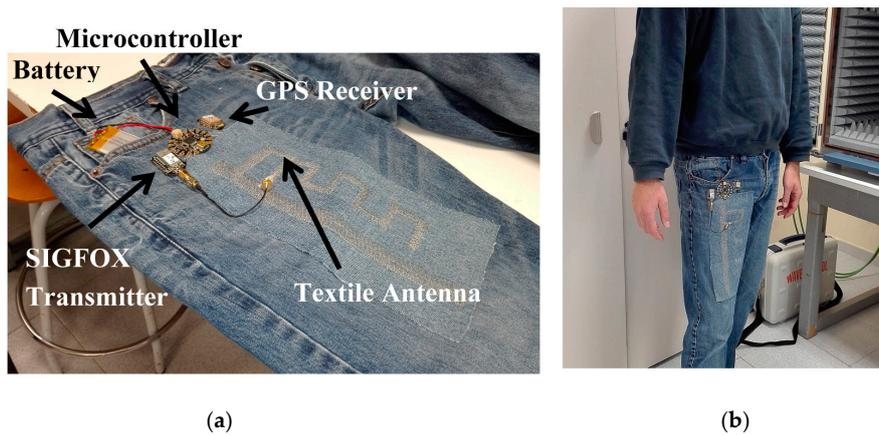
Figure 14. (a) Details of the proposed wireless wearable sensor node; (b) On-body wearable system.
