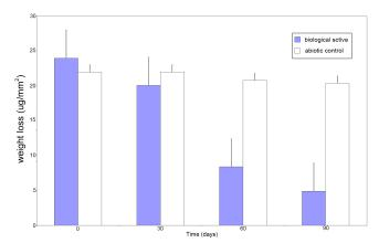
**Figure 1.** Weight loss of chemically synthesized *syn*-PHB films after exposure to a biologically active soil incubated at 35°C and the controls. The soil was kept at 60% of water holding capacity and loss of moisture was adjusted by adding sterile water every 5 days. Treatment was carried out in triplicate.
