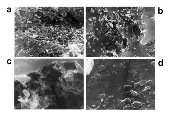
**Figure 2.** Scanning electron micrographs (SEMs) of *syn*-PHB films during incubation in a soil from biologically active flask (a,30 days; b, 60 days; c, 90 days) and from abiotic controls (d). (scale bar: a and b, 10  $\mu$ m; c and d, 5  $\mu$ m)
