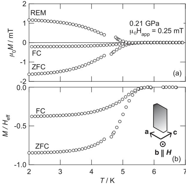
Fig. 2. (a) Magnetization vs temperature of the single crystal at 0.21 GPa for  $\mathbf{H} \parallel \mathbf{b}$ . (b) Magnetization corrected for the demagnetizing effect using  $N = 0.97$ .
