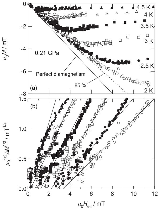
Fig. 4. (a) ZFC Low-field magnetization vs  $H_{\text{eff}}$ . Solid and broken lines denote 100% and 85% of the perfect diamagnetism, respectively. (b) Square root of the deviation from linearity (the 85% line) vs  $H_{\text{eff}}$ . Solid lines are the fit of the data to estimate  $H_{c1}$ .
