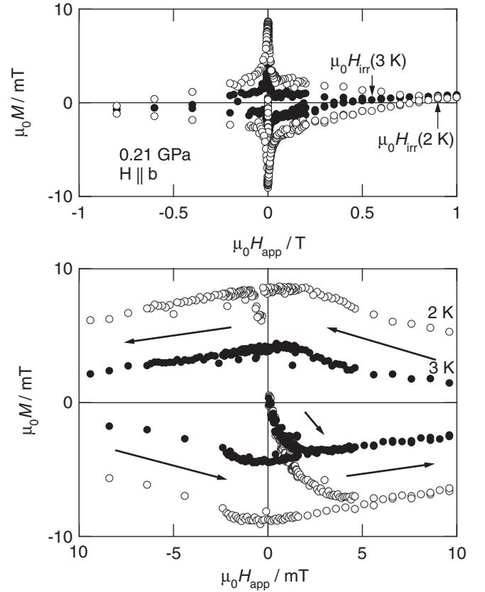
Fig. 3. Field sweep magnetization curve, showing hysteric loop behavior, taken for the single crystal at 0.21 GPa for  $\mathbf{H} \parallel \mathbf{b}$ .
