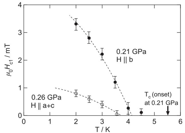
Fig. 5. Temperature dependence of  $H_{c1}$ . Dashed curves are the fit using the parabolic law below 4 K.
