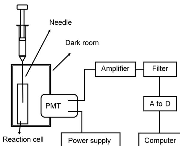
**Figure 2.** Schematic block diagram of the CL instrument. PMT: photomultiplier tube; A to D: analogue to digital converter.
