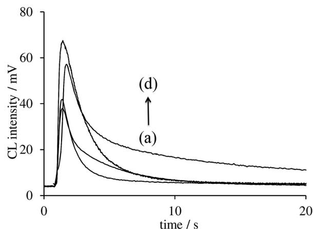
**Figure 6.** Typical CL profiles of (a) blank human plasma; (b) ascorbic acid ( $2.8 \times 10^{-5} \text{ mol L}^{-1}$ ); (c) cysteine ( $6.0 \times 10^{-5} \text{ mol L}^{-1}$ ); (d) ASA in human plasma ( $28.8 \mu\text{g mL}^{-1}$ ).
