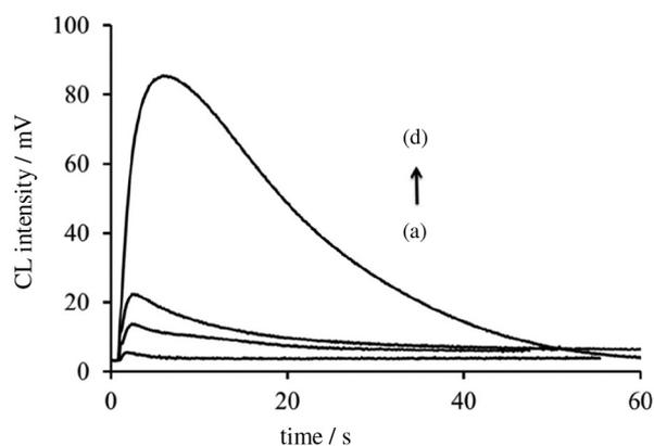
**Figure 5.** Typical CL profiles for different concentrations of ASA including: (a) blank; (b)  $14.4$ ; (c)  $28.8$  and (d)  $576 \text{ } \mu\text{g mL}^{-1}$ .
