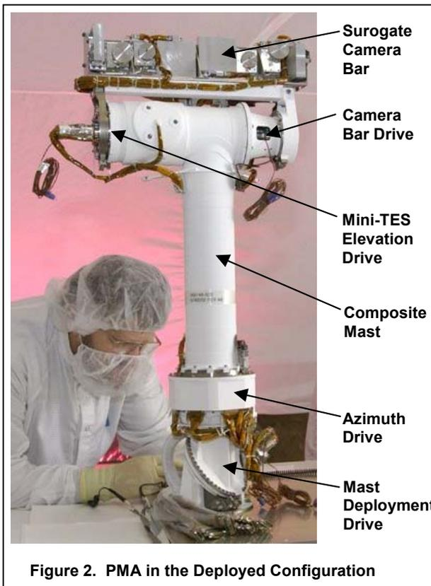
Figure 2. PMA in the Deployed Configuration
