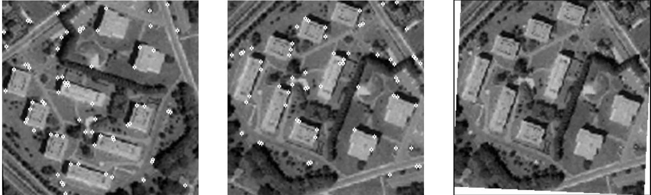
**Figure 1. Image registration using ACS Algorithm : The sensed image (left) the reference image (middle) The transformed sensed image using the best transformation found (right)**
