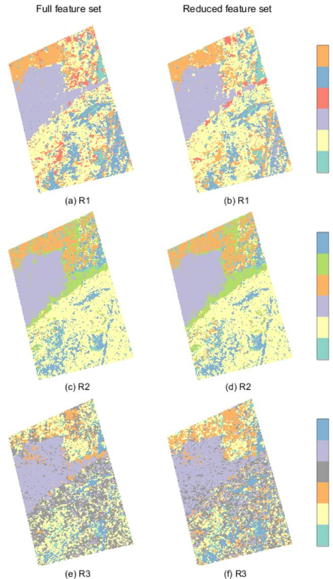
**Figure 8.** Segmentations of the three RADARSAT-2 scenes (R1, R2 and R3) into six segments. To the left: segmentation with full feature set. To the right: segmentation with reduced feature set consisting of relative kurtosis, geometric brightness, cross-polarisation ratio and co-polarisation angle.
