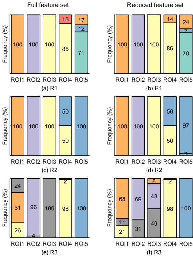
**Figure 9.** The segments assigned to the pixels in the five regions of interest by the segmentation of the three RADARSAT-2 scenes (R1, R2 and R3). To the left: segmentation with full feature set. To the right: segmentation with reduced feature set.
