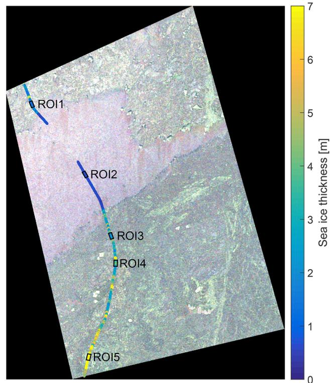
**Figure 3.** Position of regions of interest and helicopter thickness measurements displayed on the RADARSAT-2 scene from 31 August 2011 (R2). The polarimetric image is a Pauli composite, the intensity channel combinations  $|HH - VV|$ ,  $2|HV|$  and  $|HH + VV|$  are assigned to the red, green and blue (RGB) channels respectively.
