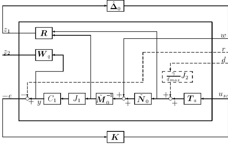
Figure 4: Generalized plant with scaled perturbation and controller for  $\mathcal{H}_\infty$  design.
