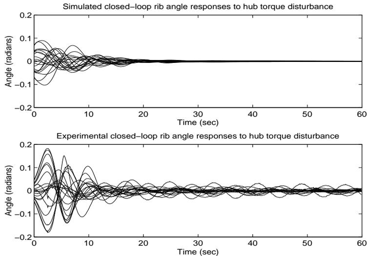
Figure 15: Simulated and experimental closed-loop rib angle responses with  $\mathbf{K}_{p2d}$ ,  $D(13.5\text{Nm}, 2s, x)$ .
