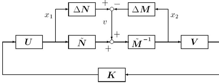
Figure 1: Feedback control of a perturbed LCF model.
