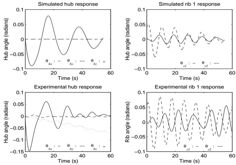
Figure 10: Simulated and experimental open-loop responses of Daisy to  $D(13.5\text{Nm}, 2s, x)$ .
