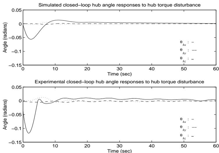
Figure 14: Simulated and experimental closed-loop hub angle responses with  $\mathbf{K}_{p2d}$ ,  $D(13.5\text{Nm}, 2s, x)$ .
