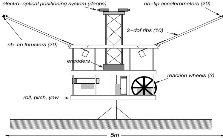
Figure 6: Daisy LFSS experimental testbed.
