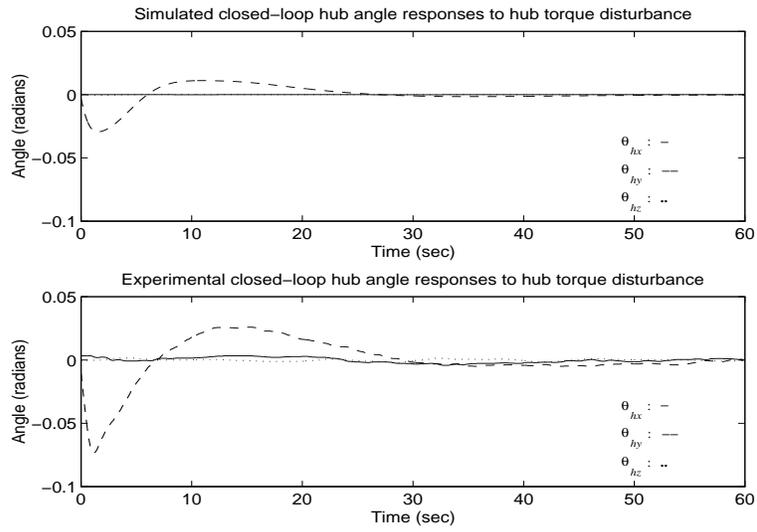
Figure 11: Simulated and experimental closed-loop hub angle responses with  $K_{p1d}$ ,  $D(13.5\text{Nm}, 2s, y)$ .
