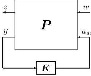
Figure 5: Generalized plant for  $\mathcal{H}_\infty$  design.
