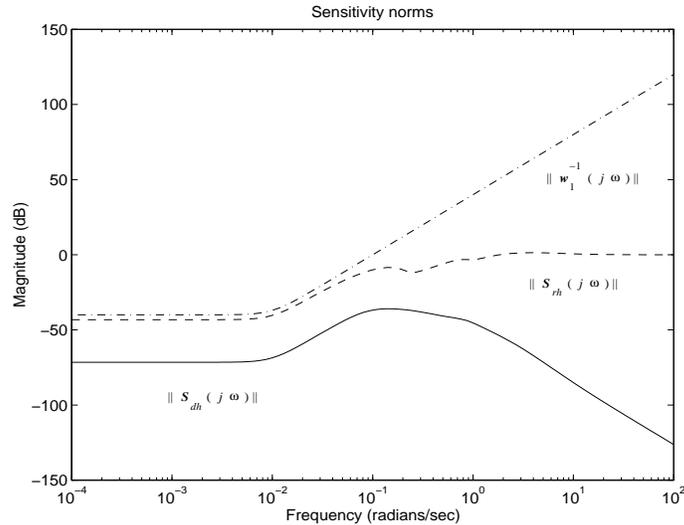
Figure 8: Norms of  $\mathbf{S}_{dh}(j\omega)$  and  $\mathbf{S}_{rh}(j\omega)$  for  $\mathbf{K}_1$ .
