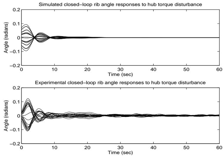
Figure 12: Simulated and experimental closed-loop rib angle responses with  $K_{p1d}$ ,  $D(13.5\text{Nm}, 2s, y)$ .
