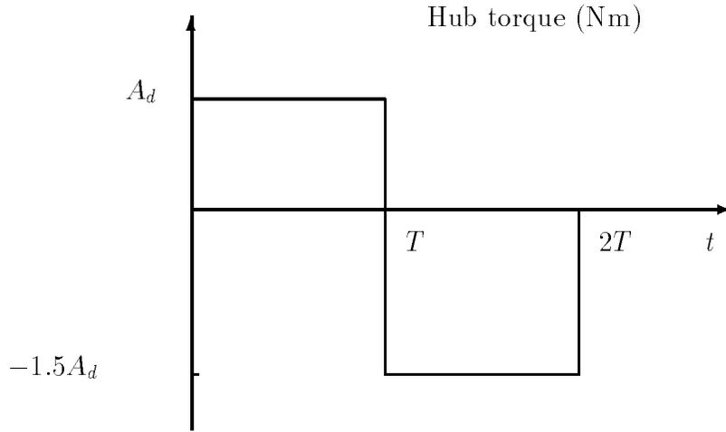
Figure 9: Standard hub torque disturbance  $D(A_d, T, axes)$
