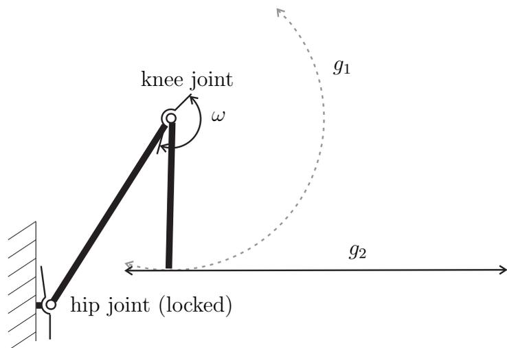
Figure 6: Actual and linearised movement of the end-effector.
