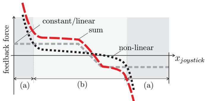
Figure 4: Adding constant/linear device-originating and non-linear kinematics-originating forces.
