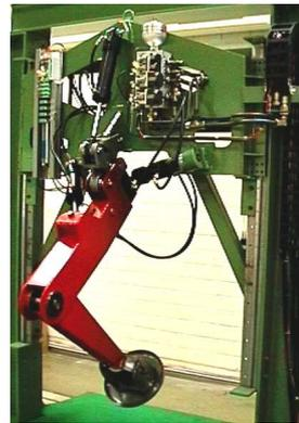
Figure 2: Leg test stand.
