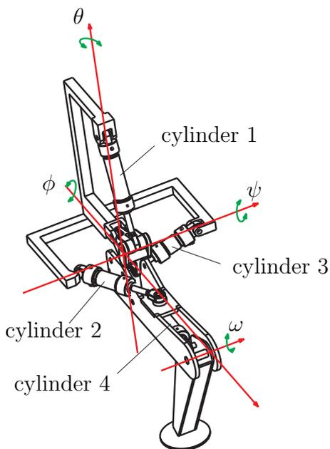
Figure 5: Kinematics of the ALDURO leg.
