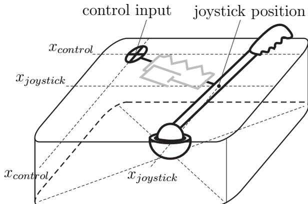
Figure 3: Virtual spring-damper system between actual joystick position and control input.
