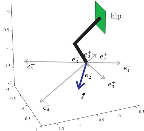
Figure 8: Vector pairs  $\{e_1\}$  to  $\{e_4\}$  and resulting repulsive force  $\mathbf{f}$
