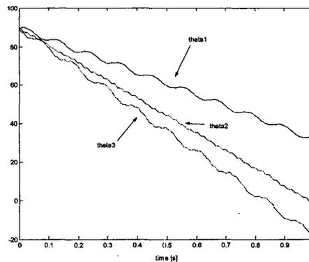
Fig. 10: Angular position of the three phalanxes (linear input:  $y_s(t) = 138.45 + 10t$ )
