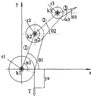
Fig. 9: Finger schematization
