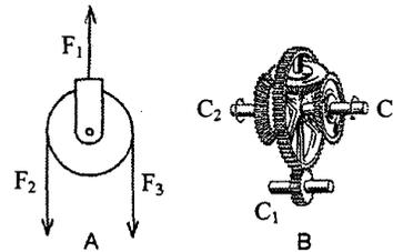
Fig. 2: Differential mechanisms: (A) movable pulley, (B) differential gear mechanism
