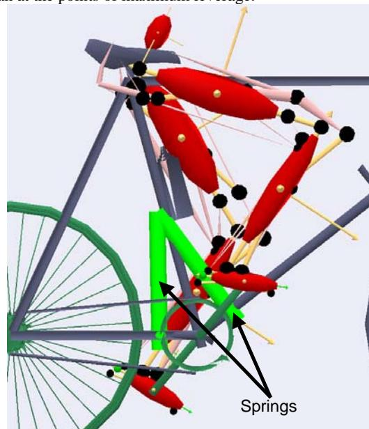
Figure 6. Placement of springs after parameter variation.
