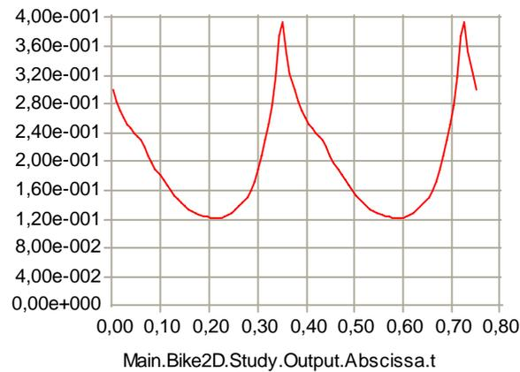
Figure 5. Maximum muscle activity over a pedal cycle at 80 rpm and constant crank moment of 30 Nm.
