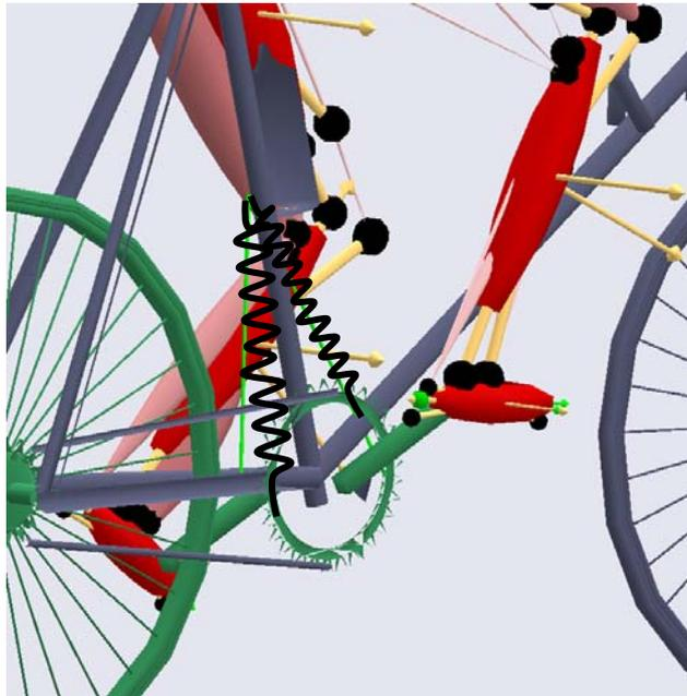
Figure 4. Two springs suspended between the frame and the chain crank mechanism.
