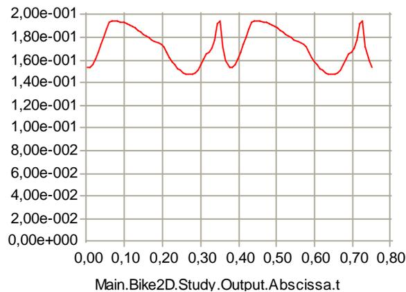
Figure 7. Maximum muscle activity over a cycle with springs added to help overcome the dead centers.
