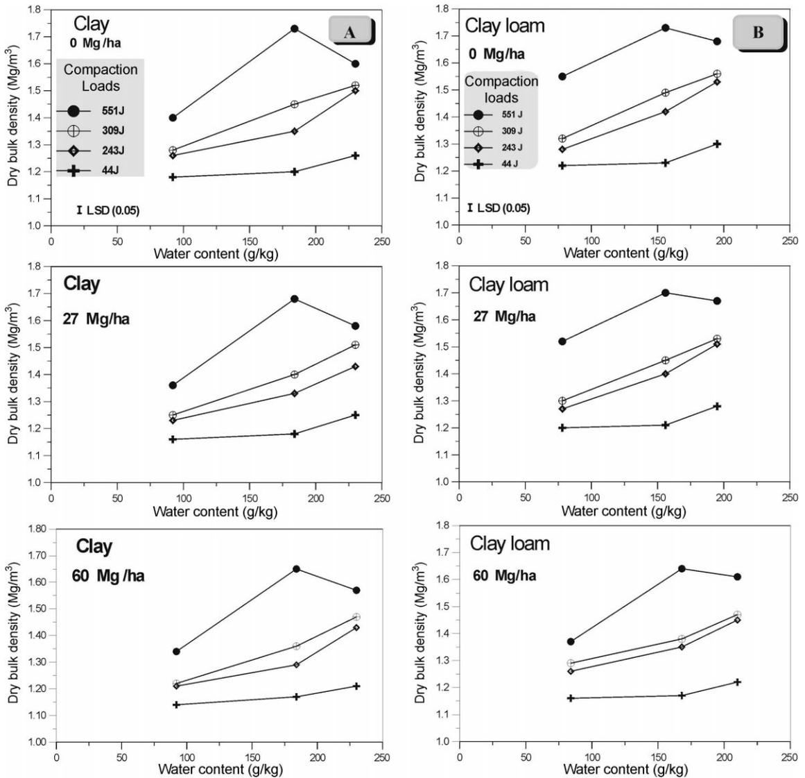
Fig. 2. Dry bulk density vs. water contents of soils at different compaction loads: A, clay soil; B, clay loam soil; C, silty clay soil. Subscripts 0, 27 and 60 refer to the amounts of incorporated sugarcane residue (Mg ha<sup>-1</sup>).
