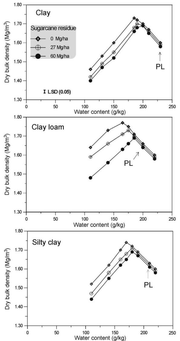
Fig. 1. Effects of water content and sugarcane residue on dry bulk density of soils using the standard Proctor test.
