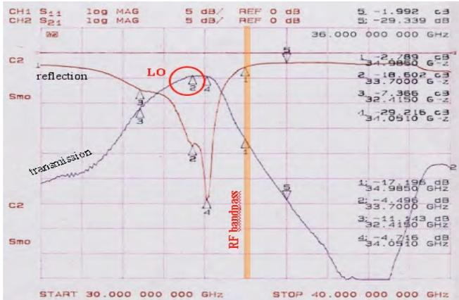
**Fig 13.** Transmission and reflection characteristics of the RF rejection filters shown in Fig 12. The plot demonstrates a 12.5 dB or better rejection in the stopband.
