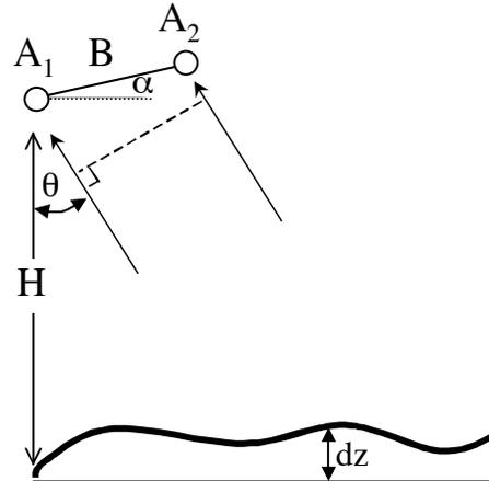
**Fig 1.** Observing geometry of a cross-track interferometric radar.
