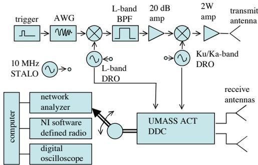
**Fig 8.** Block diagram of the full Ku-band interferometer.
