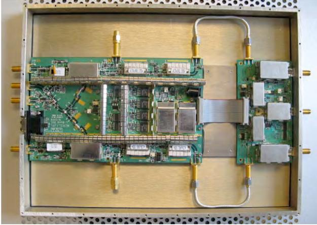
**Fig 4.** Photograph of the Ku-band downconverter in its temporary housing. The dimension of the PCB is 10"x5", which can be halved by effectively folding the PCB in two.
