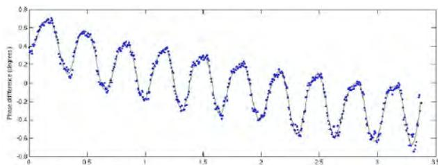
**Fig 5.** Phase difference measurements for a common signal injected into two channels of the downconverter. The plot shows the phase differences (symbols) and a low frequency curve fit to the differences. After removing the slowly varying trend (line; due to temperature changes in the room), phase measurement accuracies of 3 millidegrees can be achieved.
