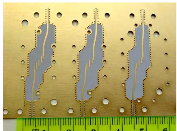
**Fig 12.** A bank of RF rejection filters constructed with small, 2.5 micron manufacturing variations meant to determine the best design for the final manufactured product.
