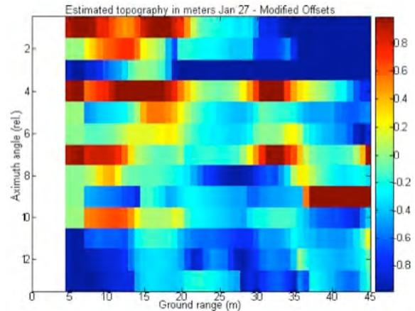
**Fig 10.** Derived topography of a snow field in Canada (2007) using the Ku-band downverter. The horizontal axis is the ground range, and the vertical axis the azimuth position. Topographic discontinuities in the above are likely due to phase wrapping occurring in single resolution elements, an effect also known as geometric decorrelation.
