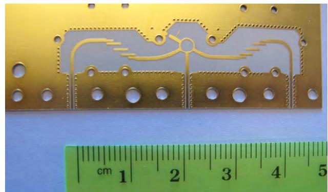
**Fig 11.** A rat-race power divider used for providing the LO signal to the two channels of downconversion. A tuning stub is provided at the difference port of the hybrid.
