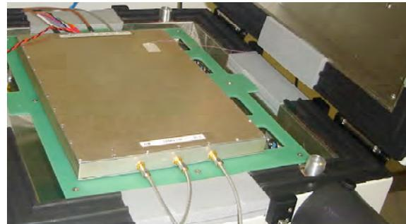
**Fig 7.** The Ku-band DDC mounted in its thermal test setup provided by the Temprotronic Corp, in Sharon, MA.
