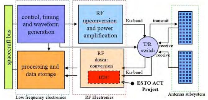
**Fig 2.** Block diagram of a microwave interferometer, highlighting the downconverter development supported by ESTO.
