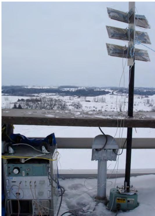
**Fig 9.** Photograph of the Ku-band interferometer deployed in Canada. Shown at left is a network analyzer data system, power supply and DDC housing, and antenna positioner control. To the right are three slot fed patch arrays, one for transmit and two for receive.
