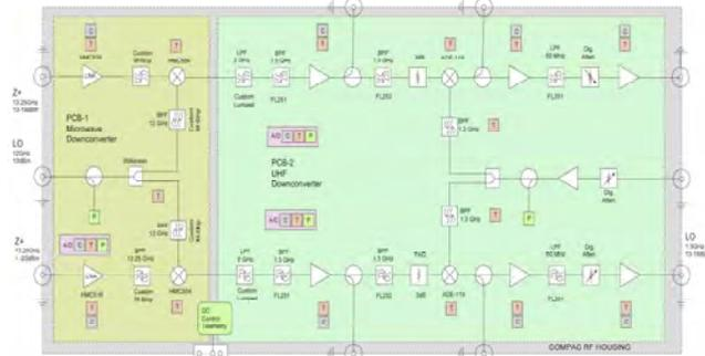
**Fig 3.** Block diagram of the two-stage, two-channel Ku-band downconverter.
