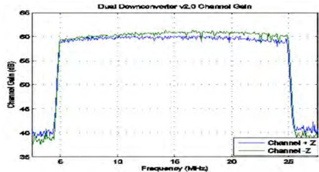
**Fig 6.** Two-channel performance over a 20 MHz bandwidth. Amplitude linearity is better than 0.2 dB, and two-channel amplitude matching is better than 2 dB.
