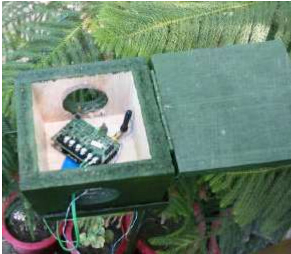
Fig. 6: Wasp-mote agriculture board along with temperature and humidity sensors
