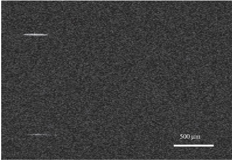
Figure 2 OCT revealed the 'glass bubble' image, an air bubble within the glass. The bubble is characterized by two parallel, bright, short lines indicating high reflectivity at the air-glass interface. However, around the sides of the bubble, light is reflected out of detection range.
