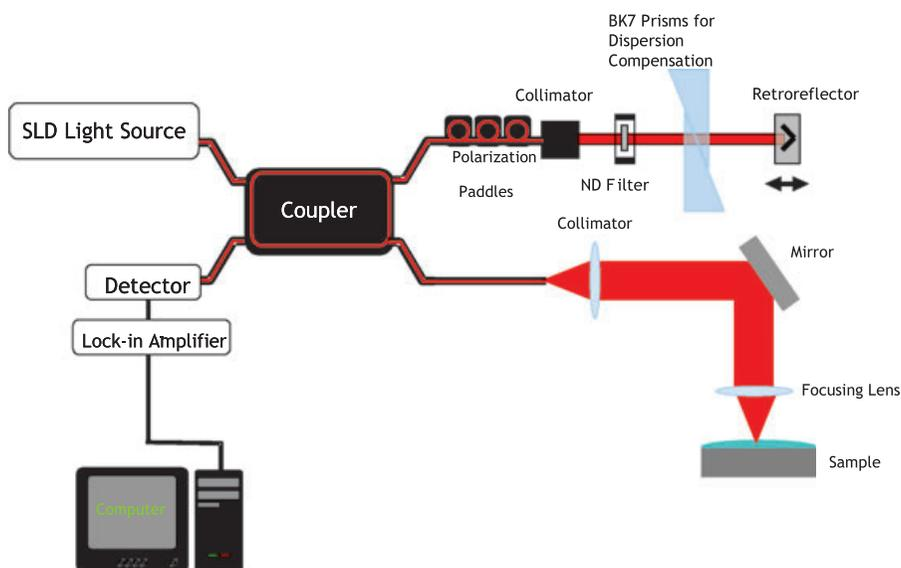
Figure 1 OCT system schematic.
