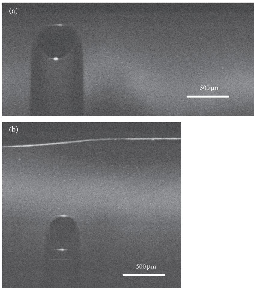
Figure 8 The two images present a bubble within a borosilicate liquid–liquid phase separated glass with light focused at different depth. Basically, the liquid–liquid phase separation background is uniform. Grey-scale variation is an artefact, due to the fixed focus of the light beam in the sample. The typical ‘l–l phase separation bubble’ with the shadowing effect is also present below the bubble.
