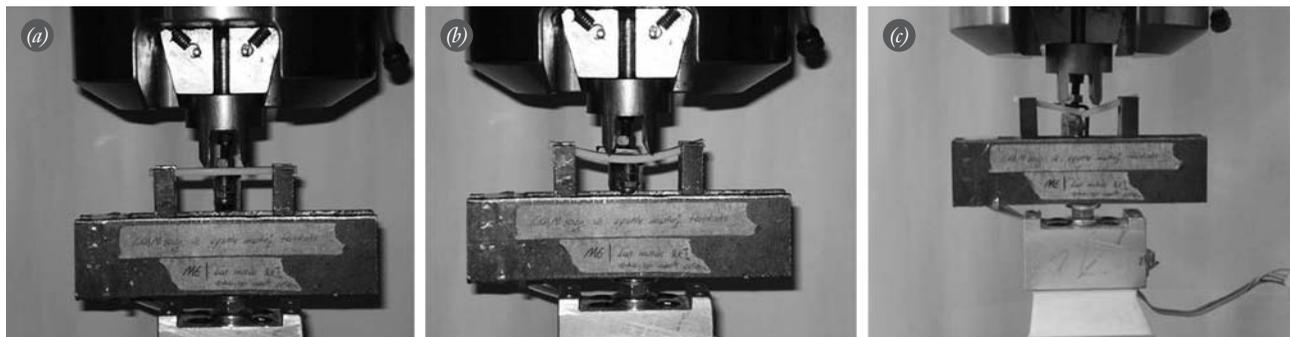
**Fig. 2.** (a-c) Figures show the bending of PMMA sample in 4-point bending test.
