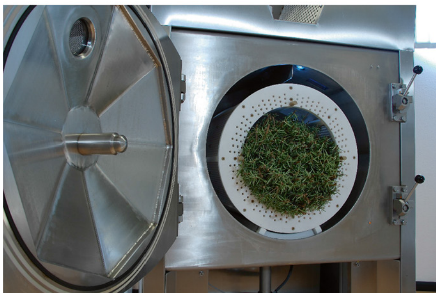
Fig. 2.3 Solvent free microwave extraction at laboratorial and industrial scale
