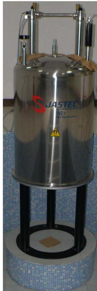
**Figure 1. Photograph of the diamagnetic levitation apparatus.** The apparatus is located in the Key Laboratory for Space Biosciences & Biotechnology of the Northwestern Polytechnical University, China. doi:10.1371/journal.pone.0024697.g001
