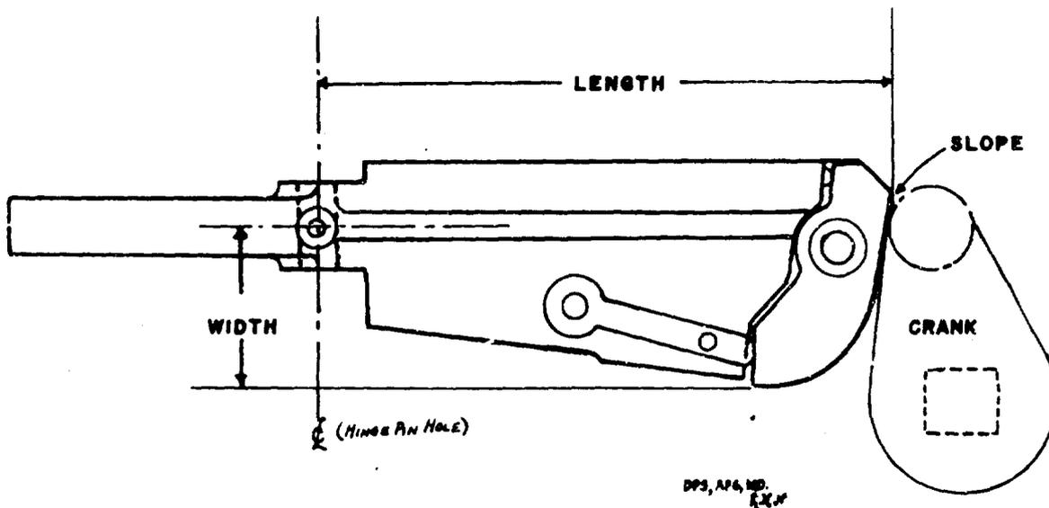
Figure A-2. Cam Critical Dimensions
