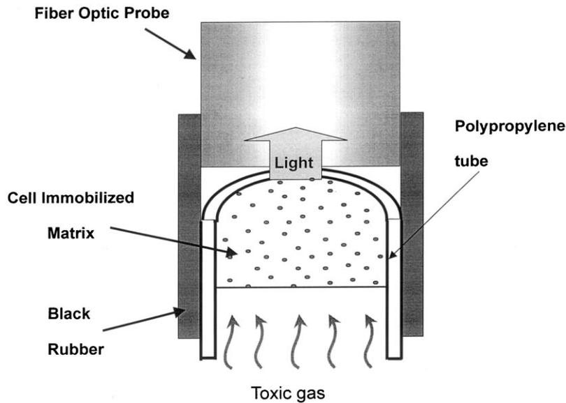
Fig. 1. Schematic diagram of the immobilized cell matrix (biosensor kit) connected with a fiber optic probe.
