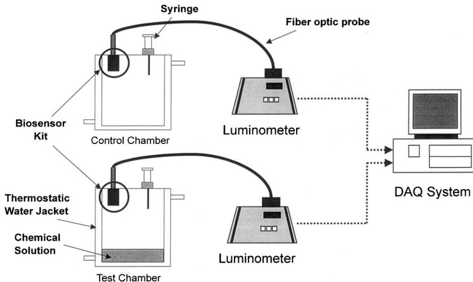
Fig. 2. BL measurement system consisting of a chamber connected with fiber optic probe and biosensor kit.
