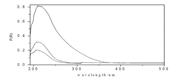
**Figure 2** Diffuse reflectantance ultraviolet-visible absorption spectra of calcined Ti-ITQ-7 with (from bottom to top) 0.15, 0.31 and 1.24 % TiO<sub>2</sub>.
