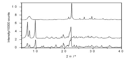
**Figure 1** X ray diffractograms of (from bottom to top) as-made and calcined Ti-ITQ-7 and as-made Ti-Beta (TiO<sub>2</sub> contents: 1.24, 1.24 and 1.40%).
