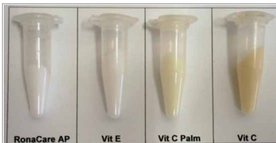
Fig. 4a Colour change of the cosmetic emulsions after 16 weeks storage at room temperature
