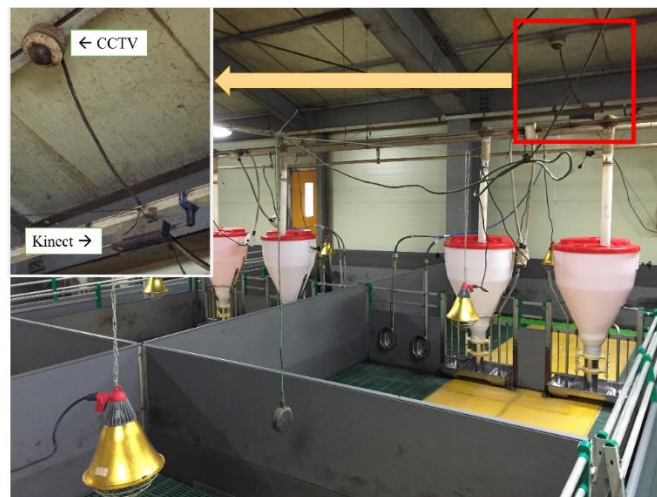
Figure 5. Pig housing unit installed with a stationary Kinect sensor.
