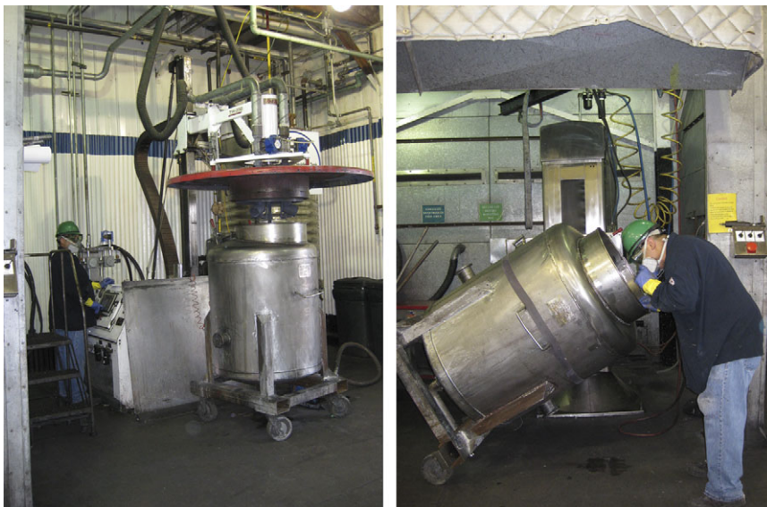
Fig. 2. Bucket-washing task (left: preparation of automatic washing of a bucket, right: checking for any residual paint left on a bucket after automatic washing).
