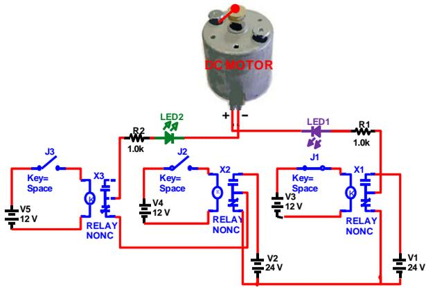
Figure 7. The drive circuit in the PIC controller experiment with the DC motor.
