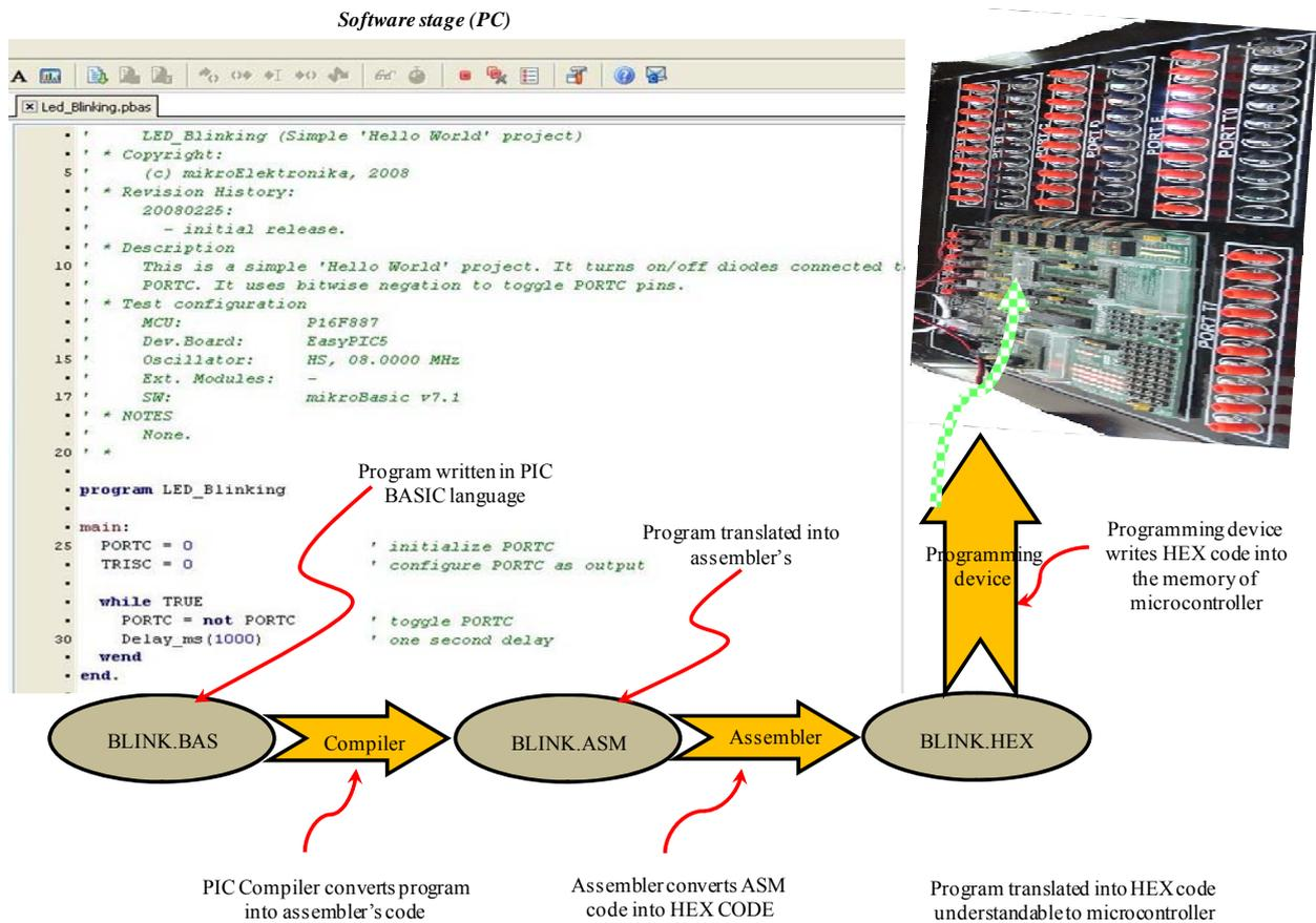
Figure 6. Details of the PIC trainer software.
