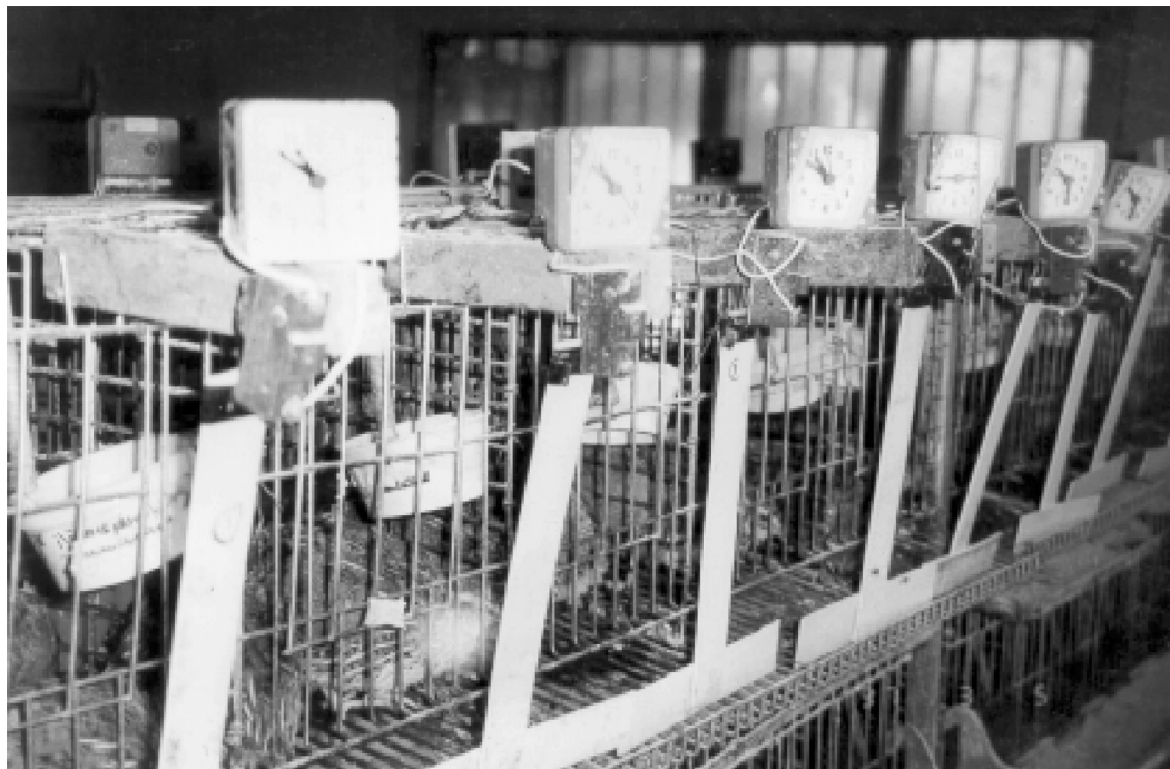
FIGURE 1. Quail breeding battery cages with oviposition detection apparatus designed to accurately detect oviposition time (Mady, 1996).
