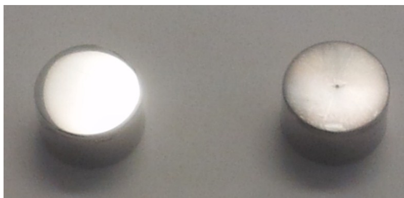
Figure S2. The surface of CoCr at OCP (left) and after application of 1V for 15 min (right).
