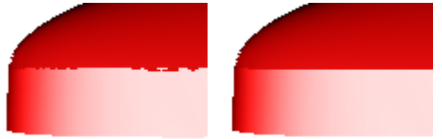
Figure 4: Left: Aliasing artifact due to partly intersecting fat borders. Right: Pushing back the fat borders reduces the artifact.
