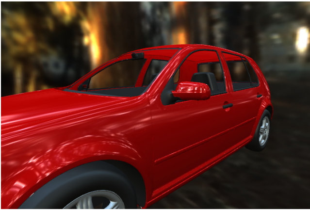
Figure 9: View-dependent rendering of a car model consisting of 8036 trimmed NURBS patches using environment mapping. The model was kindly provided by Volkswagen.
