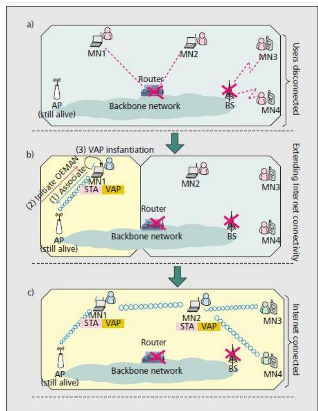
Fig 3. OEMAN establishment: a) Failure of Infrastructure; b) Extending the Internet; c) Wireless access network
