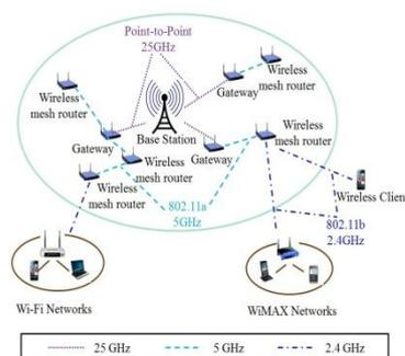
Fig 2. Internetworking Wireless Mesh Network
