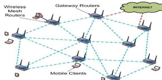
Fig 1. Basic Wireless Mesh Network infrastructure.
