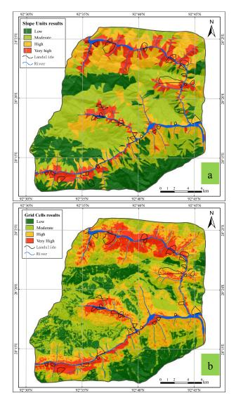
Figure 8. Landslide susceptibility map results using (a) slope units and (b) grid cells.
