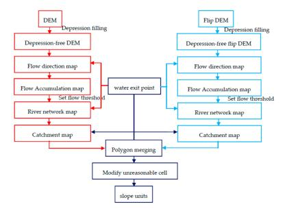
Figure 2. Construction process of the slope unit.
