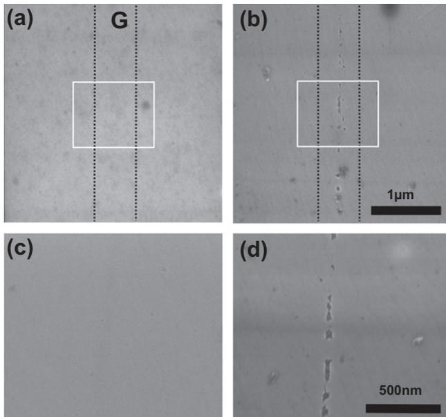
**Fig. 5.** Top-down SEM images of a stressed AlGaIn/GaN HEMT (nm-scale gate device) after deprocessing: (a) a region without detected under-gate defects, (b) a region of the same device with a distinct line of under-gate defects, (c) high-magnification view from the boxed area in parts (a) and (d) high-magnification view from the boxed area in part (b). The approximate locations of the edges of the gate (G) metalization prior to deprocessing are indicated in parts (a) and (b) (dotted lines).
