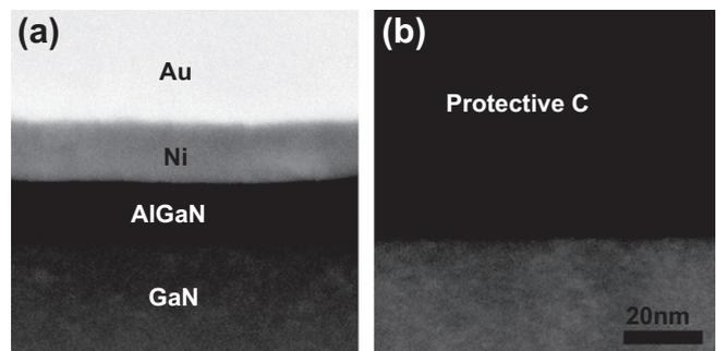
**Fig. 4.** HAADF-STEM images of the near-gate region of AlGaIn/GaN HEMTs with nm-scale gates: (a) prior to deprocessing showing the Au and Ni metal layers and (b) after deprocessing showing thorough removal of the metallization layers with the AlGaIn and GaN epilayers left completely intact. The protective C layer in (b) was deposited prior to sample preparation using focused ion beam milling to prevent surface damage.
