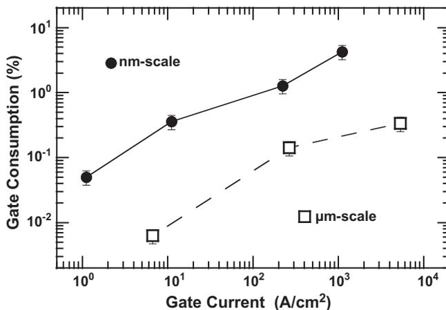
**Fig. 6.** Percentage of gate contact area consumed by under-gate defects as a function of gate leakage current density (prior to catastrophic failure) for both nm- and μm-scale devices.
